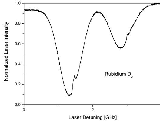
Fig. 9. Absorption profile of Rubidium.
