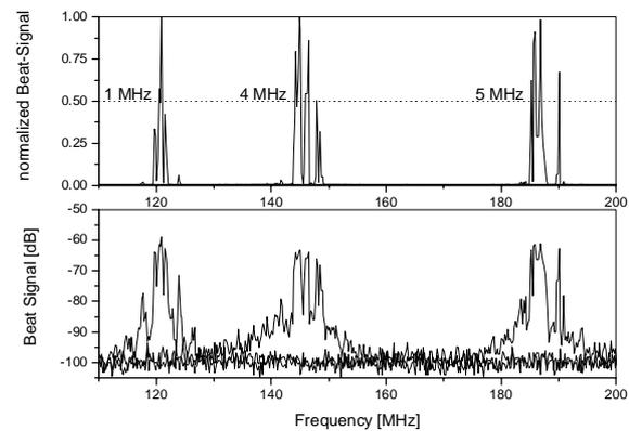
Fig. 8. Linewidth in 20 ms sweep time: < 5 MHz.
