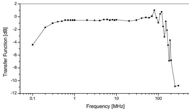
Fig. 5. Frequency response function of the current bias-tee modulation.
