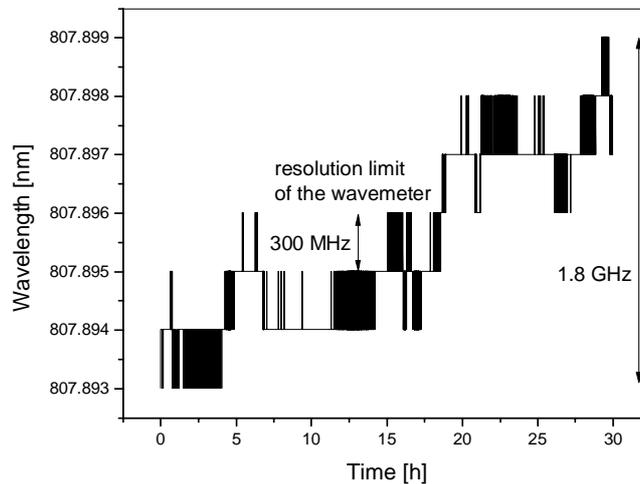
Fig.10. The wavelength of the free-running laser. The excellent thermal management of the high power ECDL ensures a drift below 2 GHz in 30 h measurement time.
