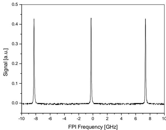
Fig. 4. Transmission of the scanning FP-cavity used to monitor the mode-hop free operation during a 15 GHz scan of the laser. Visible are the three longitudinal modes of the FPI.
