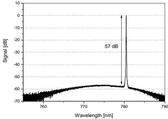
Fig. 2. Spectrum of our ECDL with a side mode suppression of 57 dB and an output power of 1 W at 780 nm.
