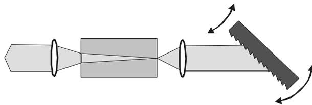
Fig. 1. The principle of the external cavity in Littrow configuration. The first order of the grating is reflected back into the diode to build the resonator. The light is coupled out of the rear facet of the diode. Wavelength tuning is achieved by moving the grating.
