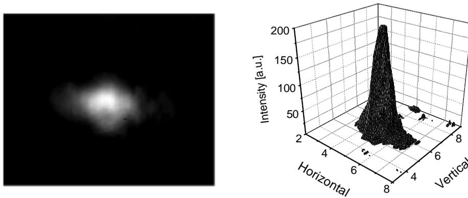
Fig. 6. The beam profile of the ECDL with an  $M^2 < 1.2$ . The fast axis is in the horizontal plane, while the slow is in the vertical.
