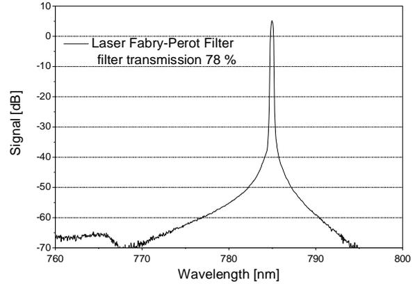
Fig. 3. Spectrum of the ECDL together with a filter resulting in a side mode suppression of 70 dB and an output power of 0.8 W at 780 nm. Peak is broadened because of the limited spectral resolution of the used analyzer system.
