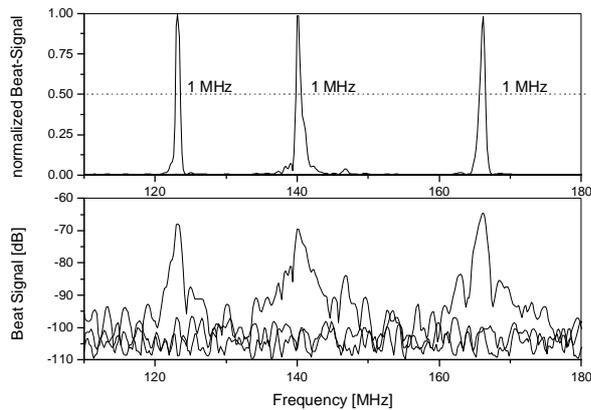
Fig. 7. Linewidth in 1 ms sweep time: 1 MHz.
