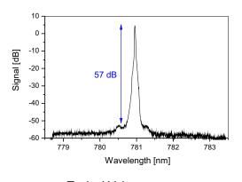
Typical Values: Power: > 1000 mW M<sup>2</sup> = 1.4 in both directions Beam Quality
