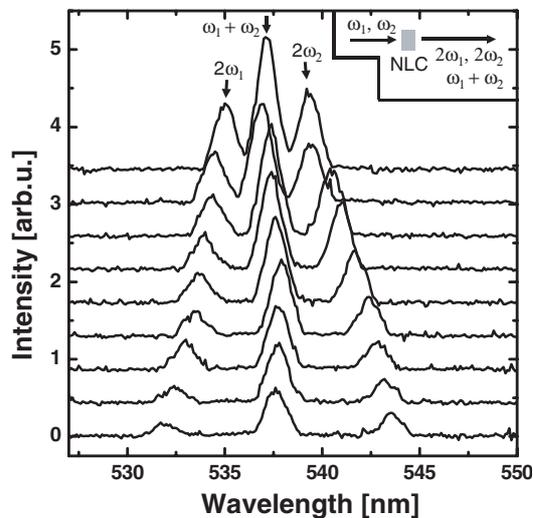
**Figure 4.** Proof of simultaneous dual-mode operation: the spectra show second harmonic signals ( $2\omega_1$ ,  $2\omega_2$ ) and a sum frequency signal ( $\omega_1 + \omega_2$ ) when the laser emission has passed a nonlinear crystal (NLC). The inset shows the scheme of second harmonic and sum frequency generation in a nonlinear crystal.
