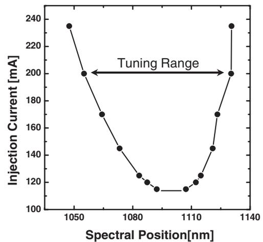
**Figure 2.** Laser threshold injection current as a function of the spectral position.
