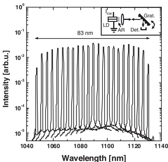
**Figure 1.** Tuning range of the QD laser in an external cavity at a bias current of 235 mA. The inset shows the experimental set-up (Littrow configuration): the laser emission of an AR coated laser diode (LD) is coupled back by the  $-1\text{st}$  order of diffraction of a grating (Grat). The  $0\text{th}$  order of diffraction is detected (Det).
